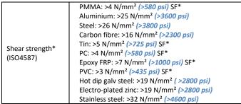
\*Strength results will vary depending on the level of surface preparation and gap. If using a cleaning solvent, allow 3-4 minutes to fully evaporate before applying adhesive. Figures above were on degreased-only substrates. SF\* = Substrate failure
