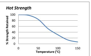
"Hot strength" shear strength tests performed on mild steel. Fully cured specimens conditioned to pull temperature for 30 minutes before testing at temperature. TA4207 can withstand higher temperatures for brief periods (such as for paint baking and wave soldering processes) providing the joint is not unduly stressed. The minimum temperature the cured adhesive can be exposed to is -40°C (-40°F) depending on the materials being bonded.
