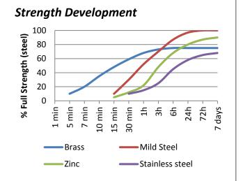
\*Cure times are typical at 23°C. Copper and its alloys will follow the faster cure while oxidised or passivated surfaces like stainless steel will tend towards the slower curve. Lower temperatures or large gaps will tend to extend the cure time. To reduce the cure time the use of Permabond A905, ASC10, or heat can be considered.
